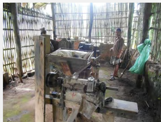
Fig 5.4.8 Rice huller integrated with IWME
