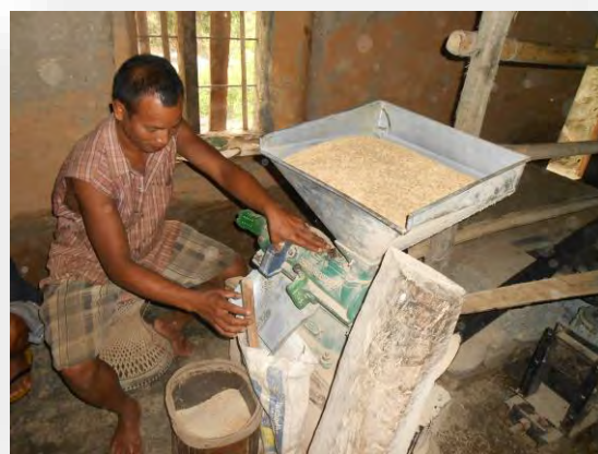
Fig 5.4.7 Paddy processing in rice huller
