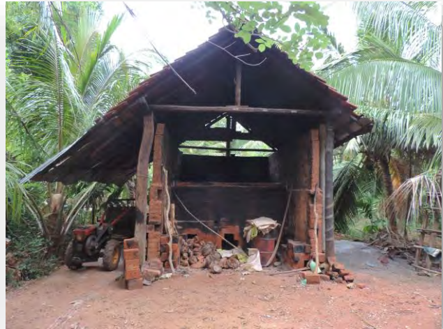
Fig 5.3.2 Dharmaratne's improved and permanent brick kiln
