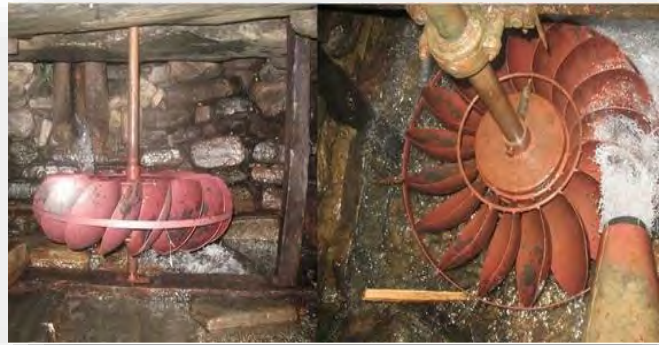
Fig 5.4.4 Improved water mill
