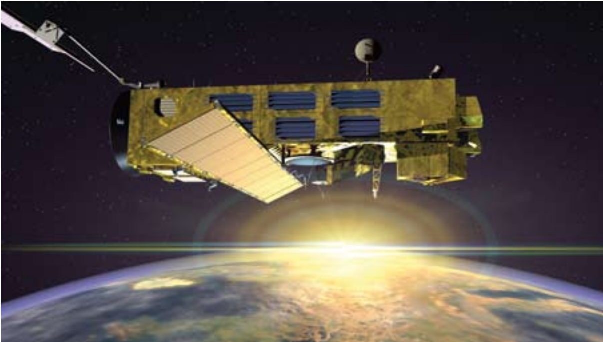
ESA Envisat, advanced polar-orbiting Earth observation satellite, which provides measurements of the atmosphere, ocean, land and ice
