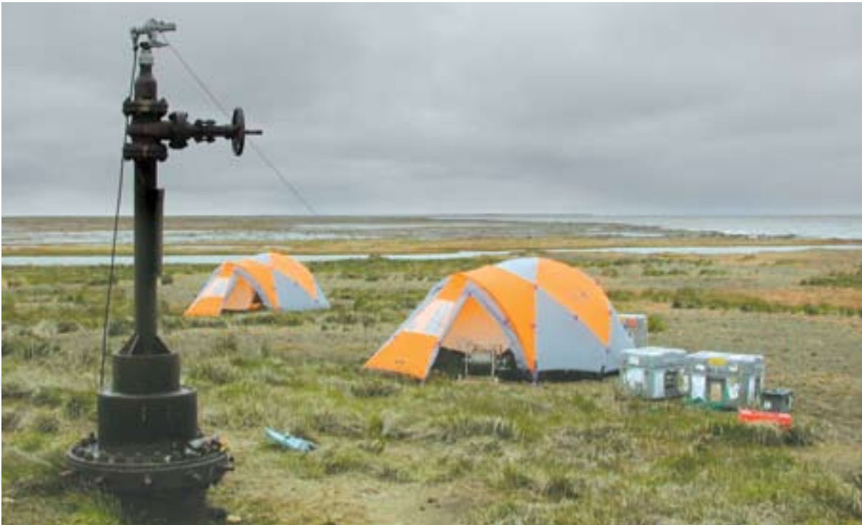
Logging permafrost temperatures in an abandoned exploratory oil well, northern Alaska. Photograph provided by Gary Clow, U.S. Geological Survey
