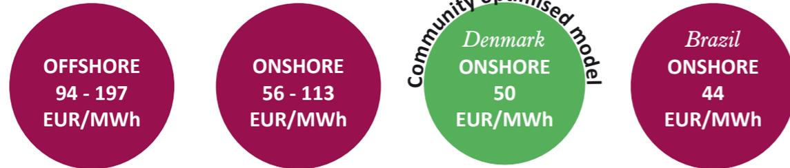
Offshore wind power has often been claimed to be the solution to avoid local protests while ensuring fulfilment of wind power implementation targets. However, economic figures show that substituting onshore capacity with offshore wind is not the right approach from society's perspective because electricity production by wind turbines is 2-3 times as expensive offshore than onshore.
