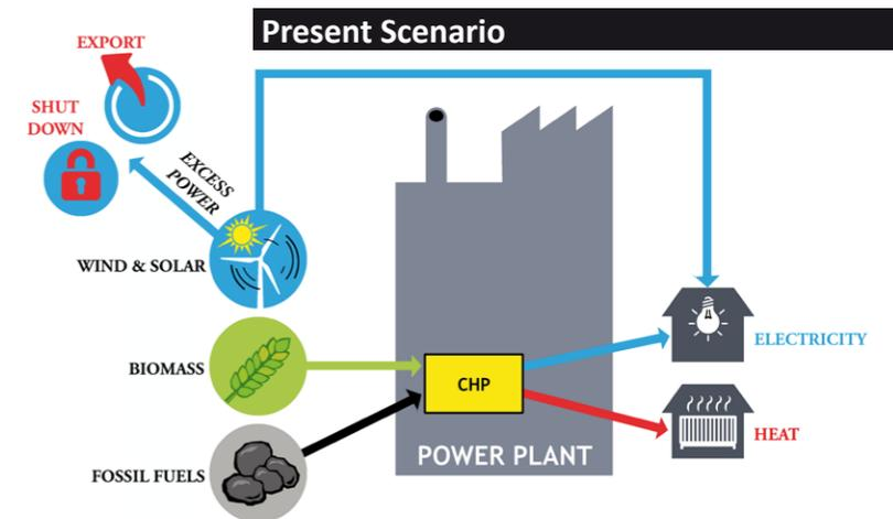
In the present scenario, wind turbines and photovoltaic panels produce electricity and combined heat and power (CHP) plants connected to district heating systems electricity and heat. All together satisfy power demand. In periods of excess power, electricity is exported or wind turbines and solar panels are shut down to keep the balance between production and demand.
