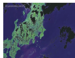
Figure 15. CAI Level 2 cloud flag for July 17, 2010, overlaid with CAI Level 1B data (see Figure 11). Black indicates clouds.
