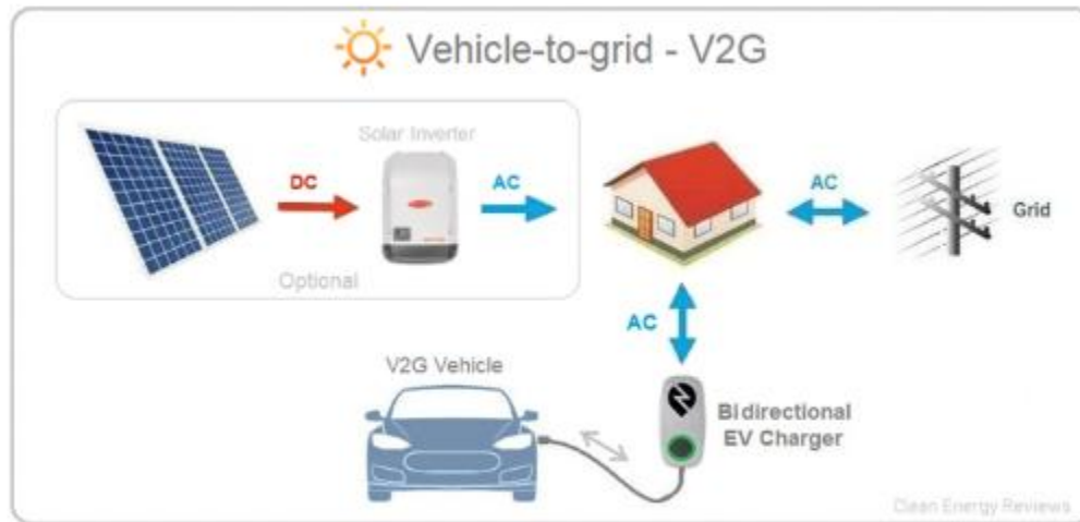
Vehicle to Grid (V2G) energy flow diagram using a DC bidirectional charger.
