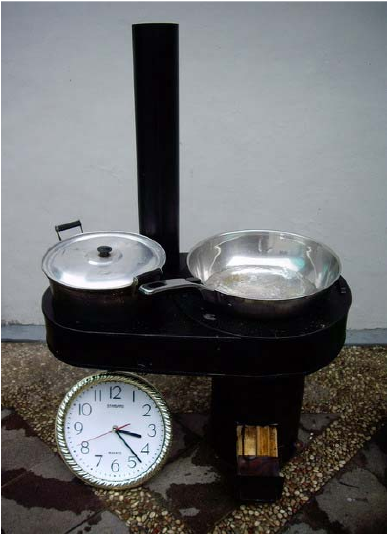
Lower fuel feed resulting in no reintroduction of smoke
