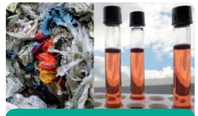
T-Technology is a system for the production of liquid fuels from the waste plastic materials. It can process the majority of plastic waste types which are normally sent to landfills, and does not require their costly preparation. One tonne of waste inputs yield 550 litres of liquid fuel.
