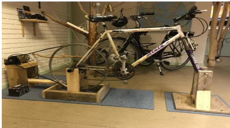
Static bike for charging power banks
