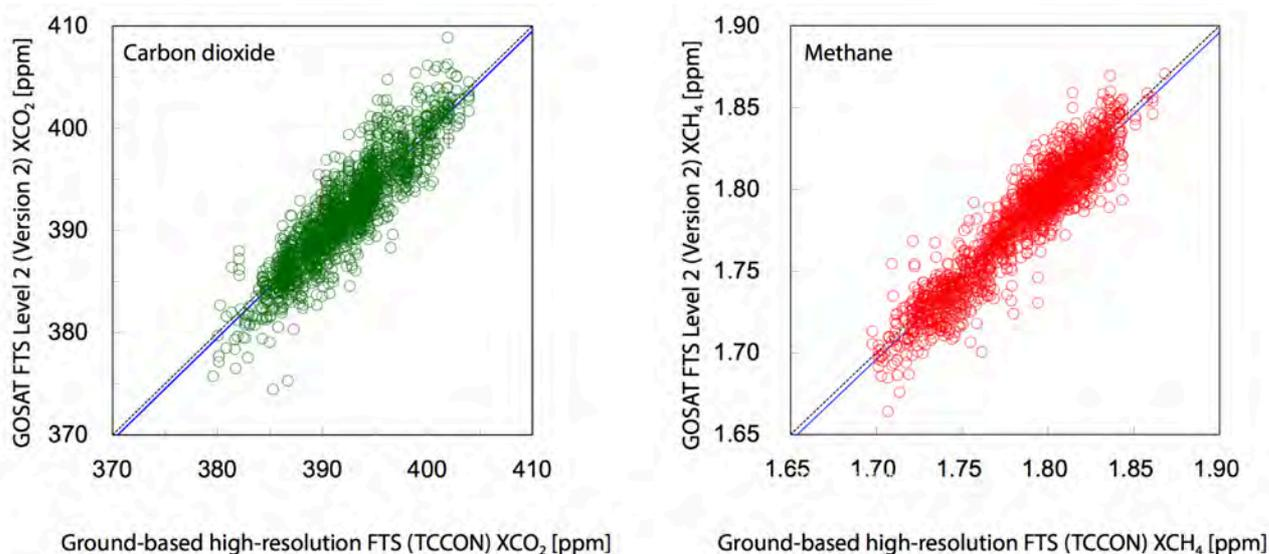
Figure 2.5-2. GOSAT FTS Level 2 products (Version 2) validation results with TCCON data:
