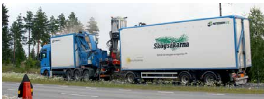
Figure 6. Chipper-truck. A system that combines chipping and transportation of forest fuel. Photo: Lars Eliasson, Skogforsk
