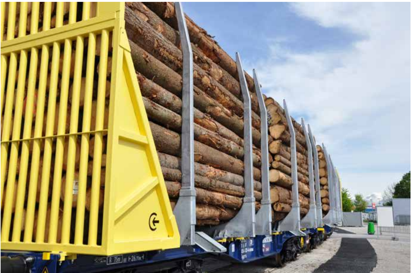
Figure 9. Optimizing the transportation of round wood is increasingly important. Innofreight designed their own stanchion system. It is a modular concept – a combination of stanchions structure and corresponding Innowagons – and is especially important and successful in the Scandinavian Region. Through the use of very wide and tall stanchion systems, the block train payload increased up to 25%. It is also possible to load pile sizes up to 34 tons (previously only 22 tons) thereby increasing cargo load and decreasing logistics costs. Other advantages include weather resistant, lower maintenance costs, faster & safer loading and unloading of wagons. Source: Innofreight
