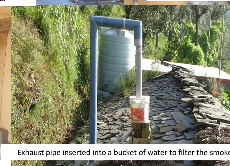
Waste heat warms the water in the tank
