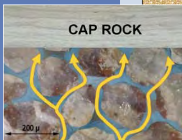
Figure 1 The injected CO 2 , which is lighter than water, tends to rise and is stopped by overlying impermeable rocks.
