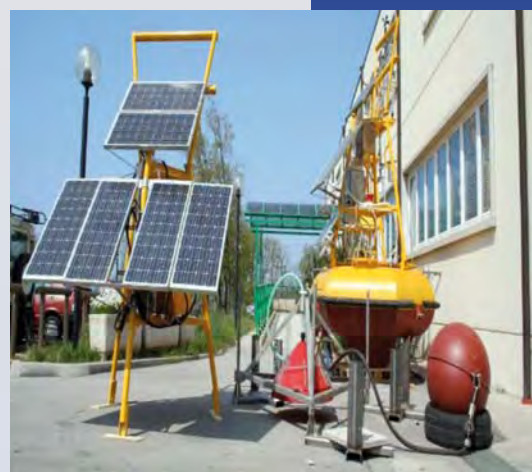
Figure 2 Monitoring buoy with solar panels for energy supply, floats and device to sample gas at the bottom of the sea.
