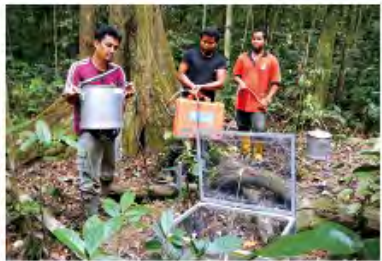
Automated chambers for soil efflux monitoring at Pasoh, Malaysia (NIES)
