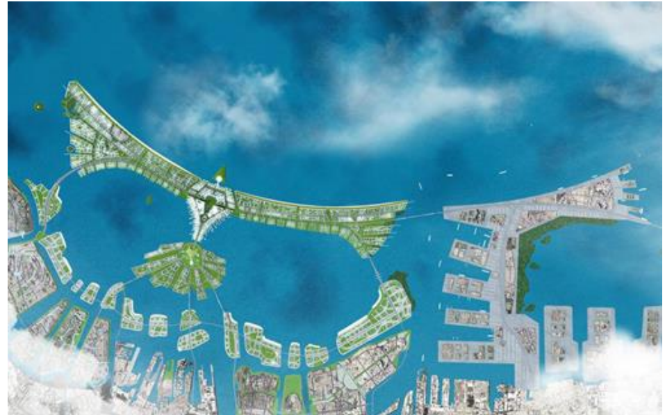
Proposed sea wall project "Garuda", 32km long x 22m tall & 17 artificial Islands
