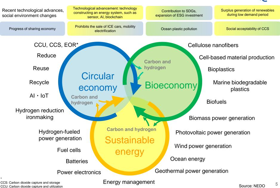
EOR: Enhanced oil recovery (injection of carbon dioxide to enhance oil production combined with CCS)
