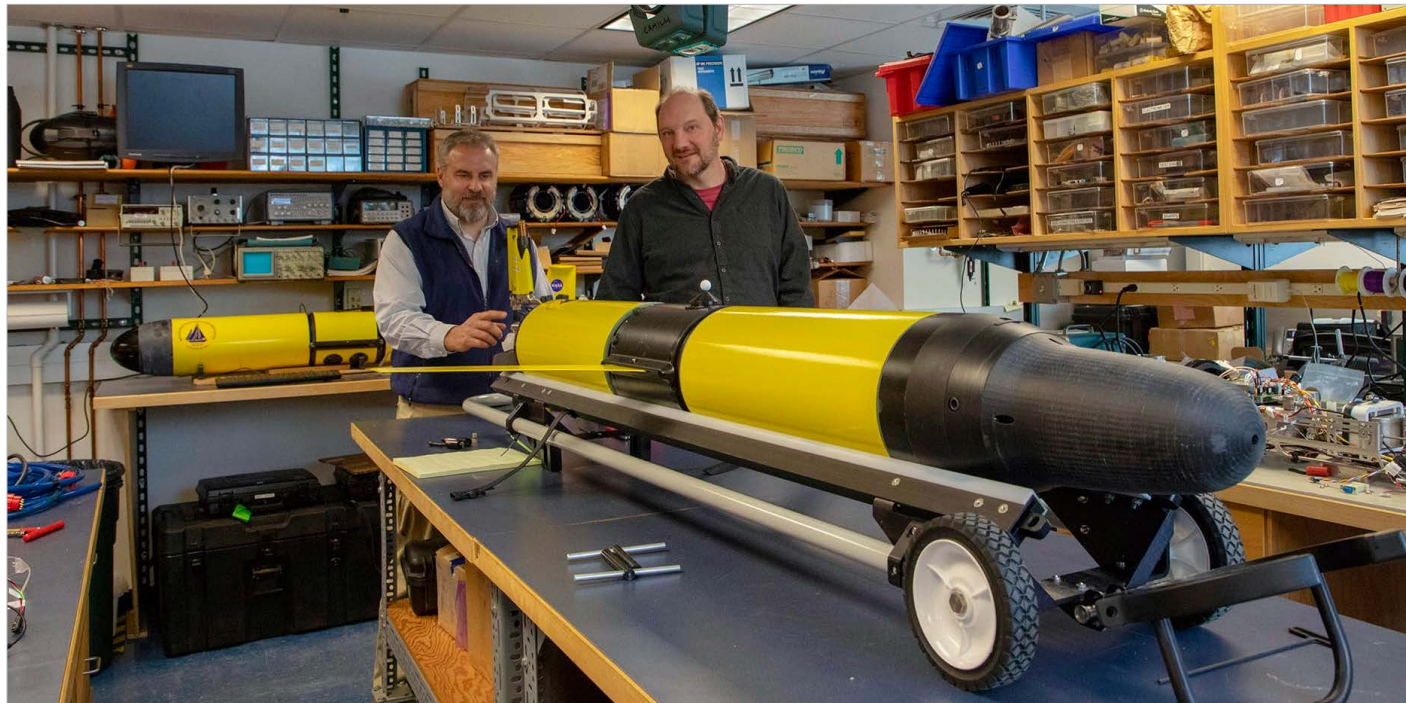
WHOI scientists Rich Camilli (left) and Ted Maksym are developing a new autonomous underwater vehicle (AUV) that will measure ice thickness from below the Arctic ocean surface for thousands of miles at a time, all with the power draw of a cell phone. (Photo by Jayne Doucette, Woods Hole Oceanographic Institution)
