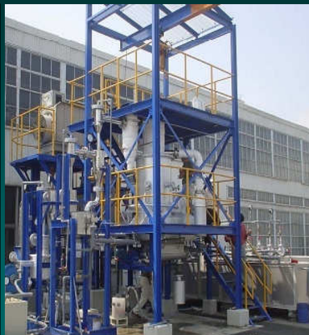
Ipalm Gasification pilot plant, Johor Capacity: 30 kW, Fuel: EFB briquettes
